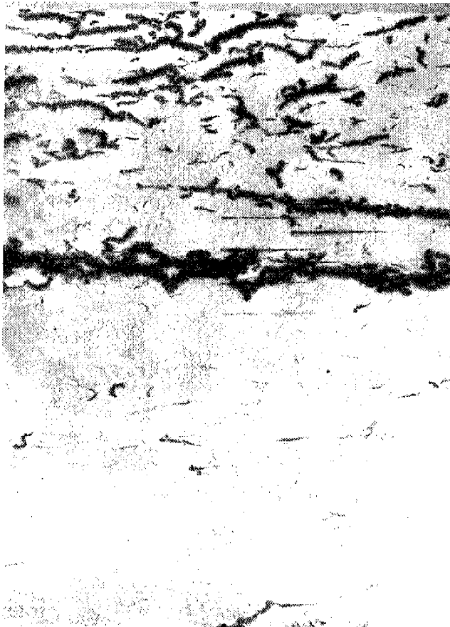
Figure 7. Photograph of stainless steel plate surface showing presence of severe slivers, laps, and ruptures.
